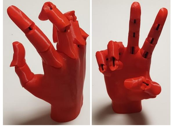
Figure 1. 3D-printed prosthetic hand
