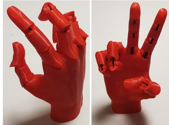
Figure 1. 3D-printed prosthetic hand
