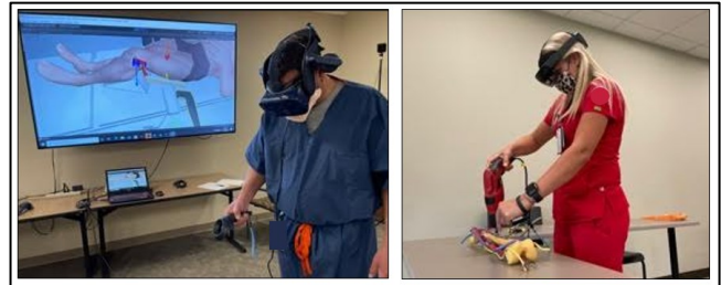
Fig. 4. Users interacting with the VR based environment using Vive Pro headset (left) and MR based environment using HoloLens 2 and physical mockup (right)
