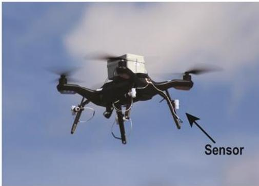
b) Dropsonde deployed from UAS
