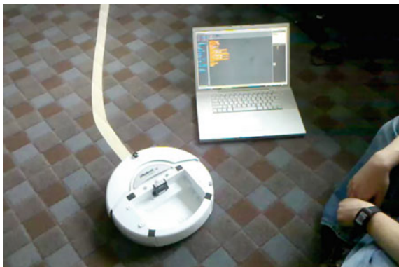
Fig. 4 Robotic control using the Scratch educational programming environment
