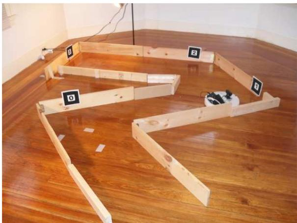
**Figure 11: A robot picks its way through a different maze from the one it was taught to navigate.**
