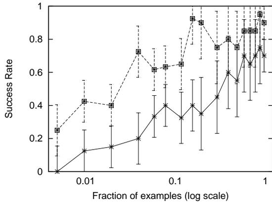
**Figure 10: Robot performance as a fraction of training trials seen. Top line represents a robot trained on tag-only data; bottom line is a robot trained by people with access to video. 1320 total trials.**
