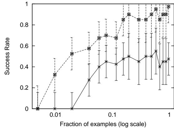
**Figure 12: Robot performance in a new, unlearned environment, as a function of the fraction of training trials seen. As in Figure 10, top line represents tag training data, bottom line is video. 900 total trials. New maze environment shown in Figure 11.**
